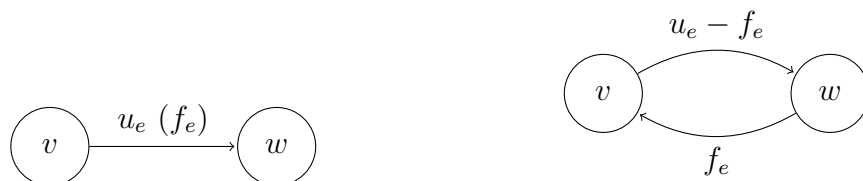
Figure 1: (a) original edge capacity and flow and (b) resultant edges in residual network.
