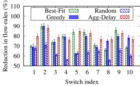
Figure 9: Reduction in flow-rules at each switch with 200 flows in the network
