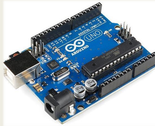
Arduino Uno based on ATMEGA328
