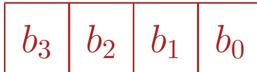
$b_3$  is zero (0) for a positive number and it is one (1) for a negative number. Other three bits  $b_2 b_1 b_0$  represent the magnitude of the number.
