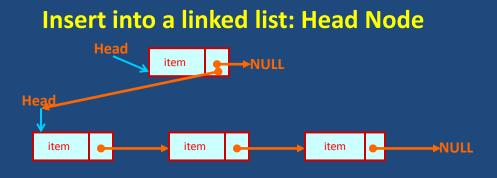
Step 4ci: Make the next of new node as the address of existing head node.Step 4cii: Copy the address of the new node as the head node.
