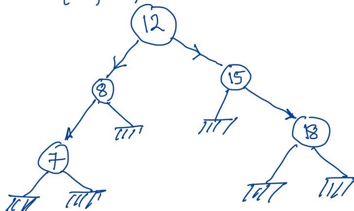
Height Balanced BST that minimizes the length of the longest path is optimal in the worst case.
