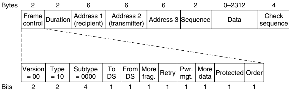
Figure 4-29. Format of the 802.11 data frame.
