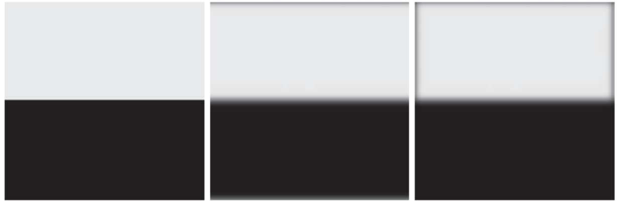
FIGURE 4.31 (a) A simple image. (b) Result of blurring with a Gaussian lowpass filter without padding. (c) Result of lowpass filtering with zero padding. Compare the vertical edges in (b) and (c).
