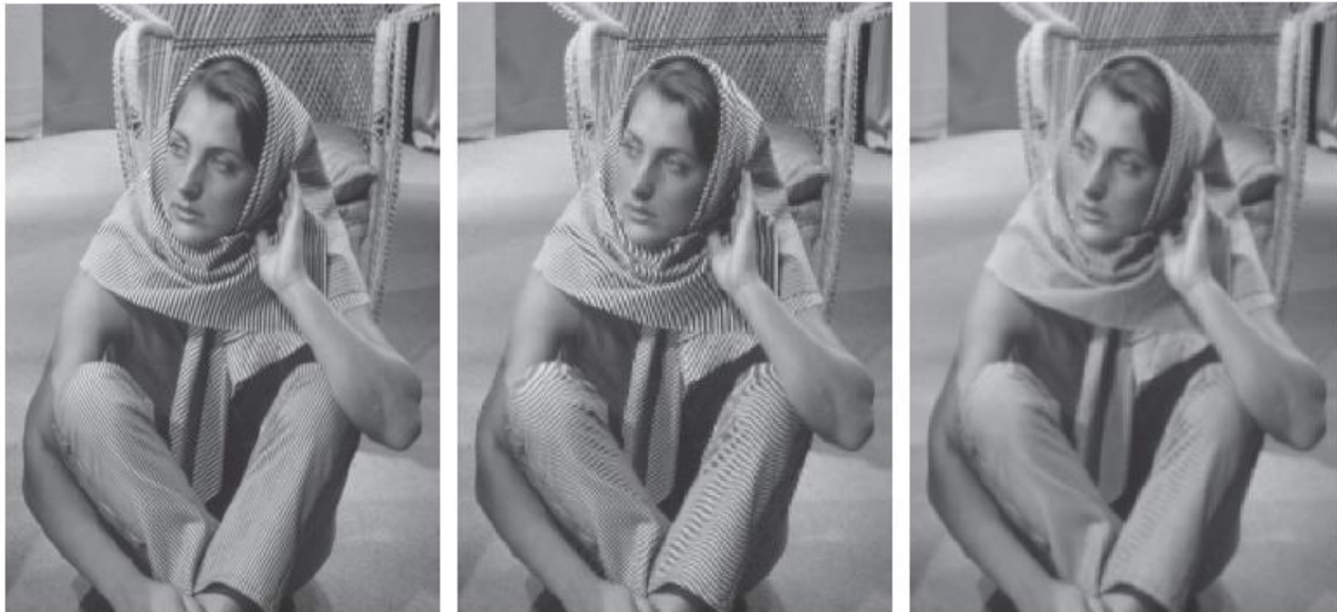
FIGURE 4.19 Illustration of aliasing on resampled natural images. (a) A digital image of size 772 \times 548 pixels with visually negligible aliasing. (b) Result of resizing the image to 33% of its original size by pixel deletion and then restoring it to its original size by pixel replication. Aliasing is clearly visible. (c) Result of blurring the image in (a) with an averaging filter prior to resizing. The image is slightly more blurred than (b), but aliasing is not longer objectionable. (Original image courtesy of the Signal Compression Laboratory, University of California, Santa Barbara.)
