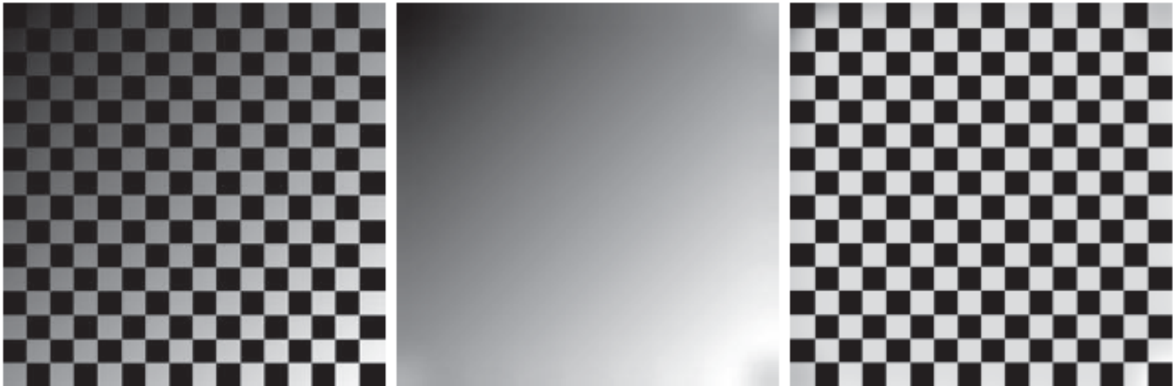
FIGURE 3.42 (a) Image shaded by a shading pattern oriented in the -45^\circ direction. (b) Estimate of the shading patterns obtained using lowpass filtering. (c) Result of dividing (a) by (b). (See Section 9.8 for a morphological approach to shading correction).
