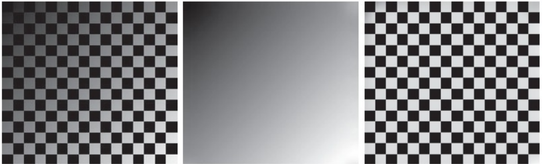
FIGURE 2.33 Shading correction. (a) Shaded test pattern. (b) Estimated shading pattern. (c) Product of (a) by the reciprocal of (b). (See Section 3.5 for a discussion of how (b) was estimated.)
