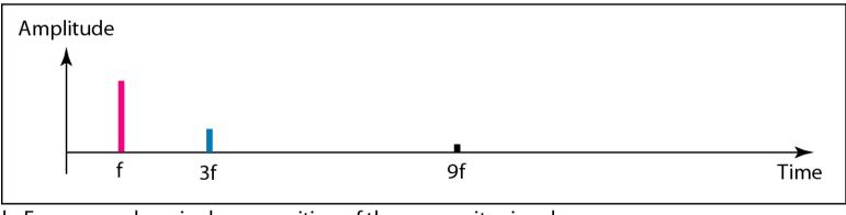
b. Frequency-domain decomposition of the composite signal
