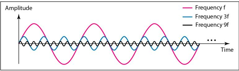
a. Time-domain decomposition of a composite signal
