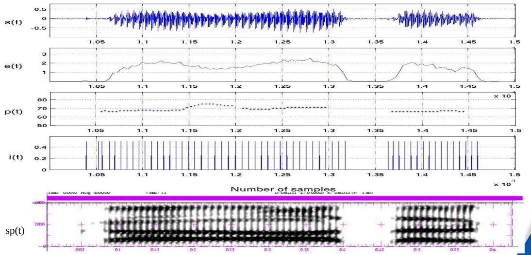
s(t): speech waveform, e(t): energy contour, p(t): pitch contor, i(t): instants of significant excitation and sp(t) : spectrogram
