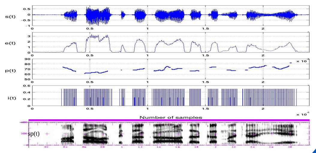
s(t): speech waveform, e(t): energy contour, p(t): pitch contour, i(t): instants of significant excitation and sp(t) : spectrogram
