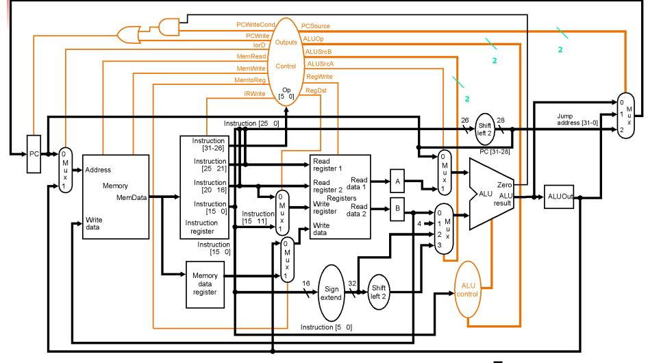
Note the reason for each control signal; also note that  $w \overline{\phi}$  have included the jump
