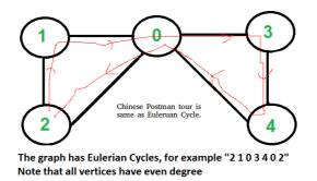
Note: It doesn't matter whether the graph is weighted or unweighted, the Chinese Postman Route is always the same as Eulerian Circuit if it exists. In the weighted graph, the minimum possible weight of the Postman tour is the sum of all edge weights which we get through the Eulerian Circuit.
