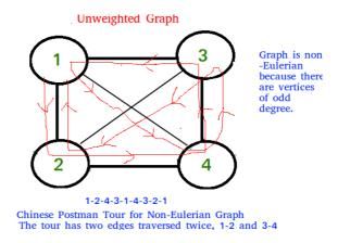
Case 3: The input graph does not contain an Euler circuit; however it can be converted to a graph with an Euler circle.
