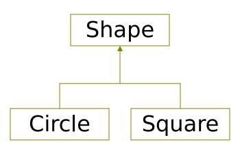
This is an Object-oriented program for graphical tool. Two shapes are there: circle, square. Each have functions draw(), rotate(), move()
