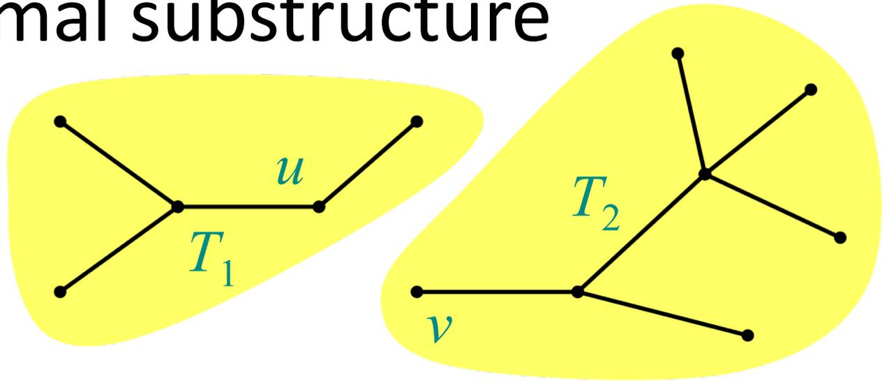
Remove any edge  $(u, v) \in T$ . Then,  $T$  is partitioned into two subtrees  $T_1$  and  $T_2$ .
