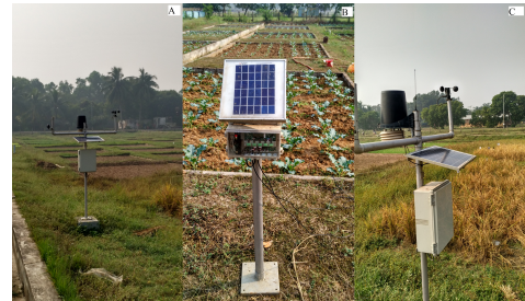
Figure 3: Our implemented agricultural IoT slave nodes. (A) Weather station, (B) Soil sensor node, (C) Weather station.
