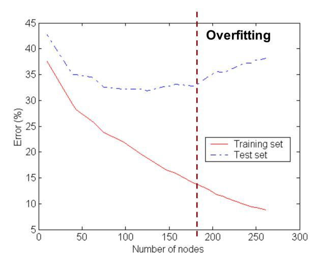
**Underfitting**: when DT is too simple, both training and test errors are large **Overfitting**: DT has grown too large, and is now fitting the noise in the dataset
