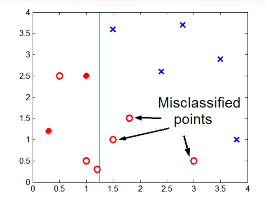
Lack of data points in the lower half of the diagram makes it difficult to predict correctly the class labels of that region
