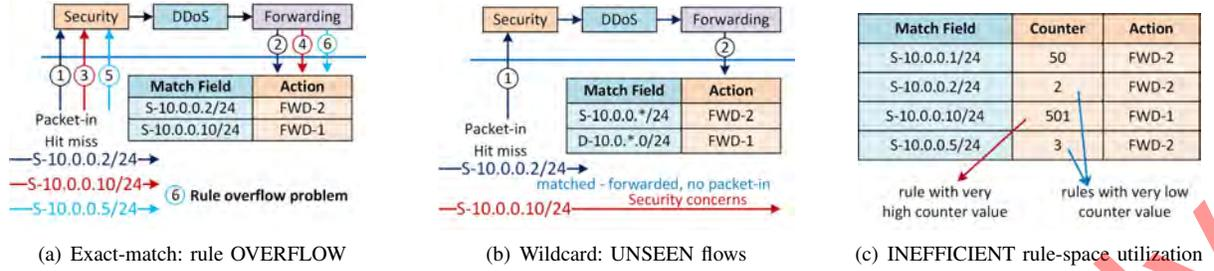
Fig. 1: Issues in TCAM-based rule placement in SDN
