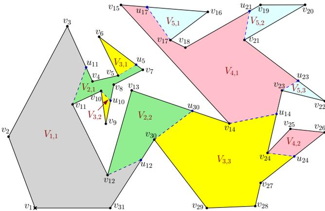
Fig. 6. Figure showing the partitioning of a simple polygon into visibility windows.
