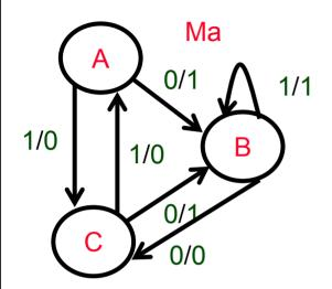
If an input sequence X takes a machine from a state Si to Sj, then Sj is said to be the X-successor of Si.
