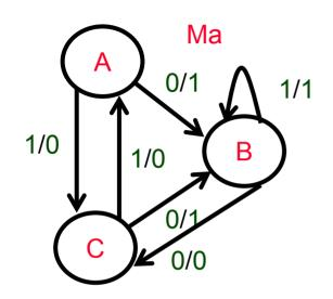
If there exists for pair (Si,Sj), a distinguishing sequence of length k, the states in (Si,Sj) are said to be k-distinguishable.
