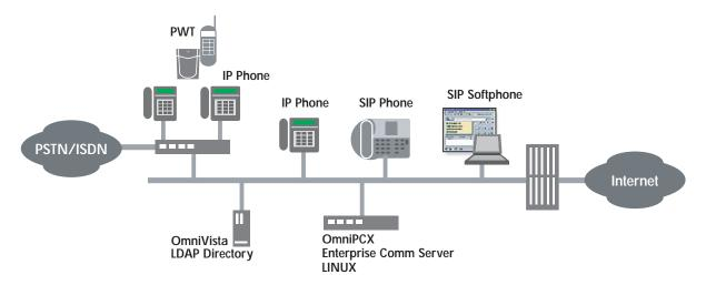
SIP is also a signaling component in Alcatel's e-Communications Center environment, which combines unified messaging, personal information management, personal routing management and Web-enabled soft phone capabilities. SIP and RTP ensure the signaling connection from the OmniPCX Enterprise to the Media Server, which drives the SIP user agent and VxML functions.
