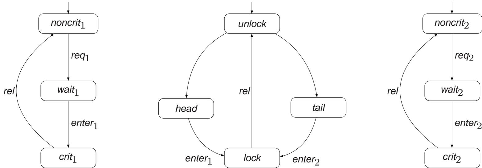
$$TS_1 \parallel \text{Arbiter} \parallel TS_2 \not\models (\forall \square \forall \diamond \text{crit}_1) \wedge (\forall \square \forall \diamond \text{crit}_2)$$
