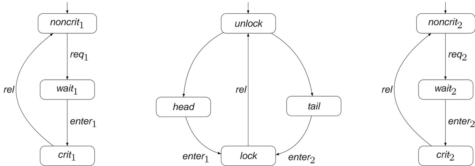
$$TS_1 \parallel \text{Arbiter} \parallel TS_2 \not\models \square \diamond \text{crit}_1$$
