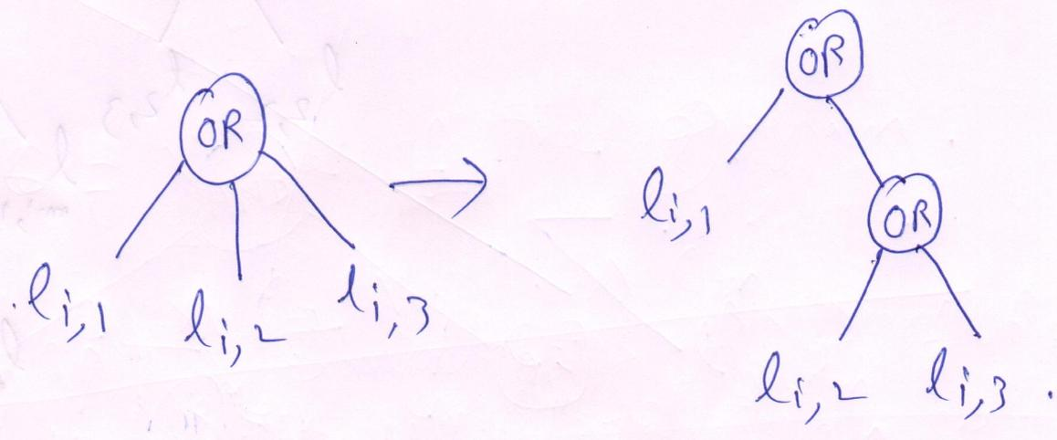
Finally, replace the top AND by the following Boolean circuit.
