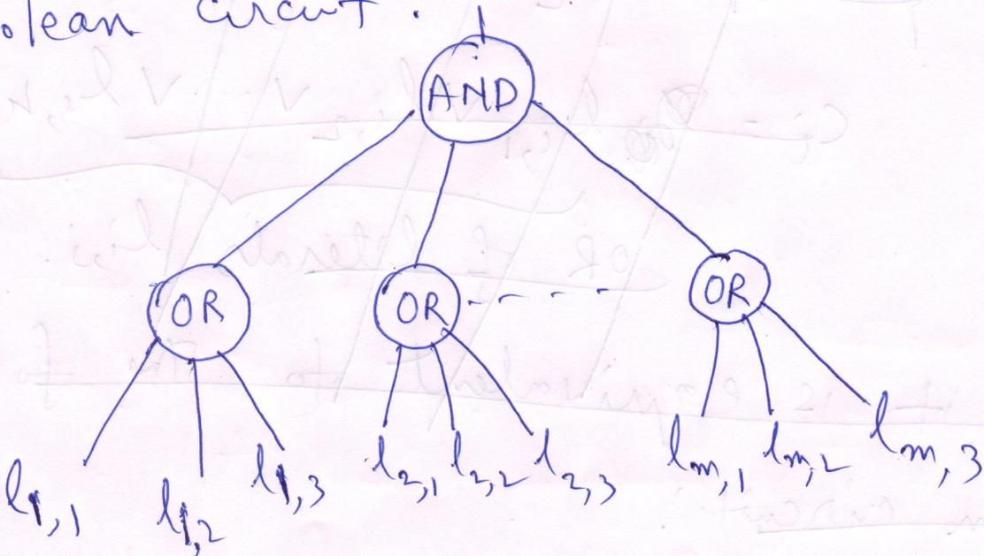
But in a Circuit-Sat instance, the AND and OR gates need to be binary / 2-input / fan-in 2. Thus replace each of the bottom ORs by a two level circuit with binary OR!
