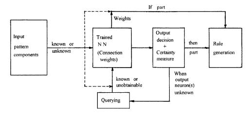
Fig. 3. Block diagram of inferencing and rule generation phases.
