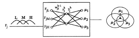
Fig. 2. Block diagram of a fuzzy neural network.
