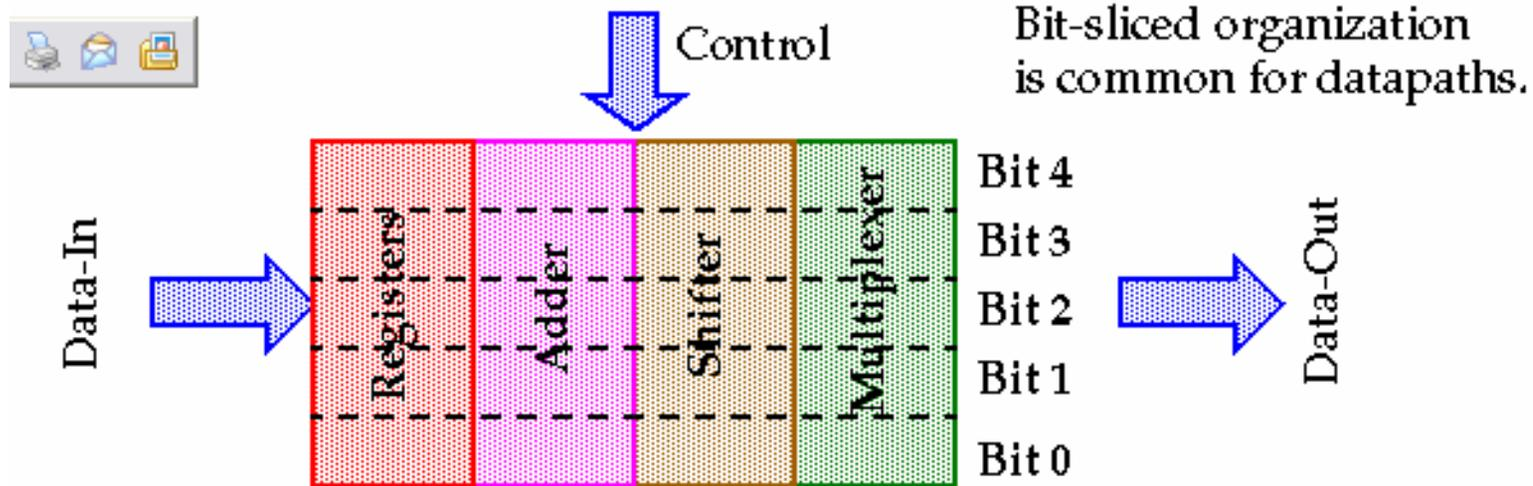
*How can we develop architectures which are bit sliced?*
