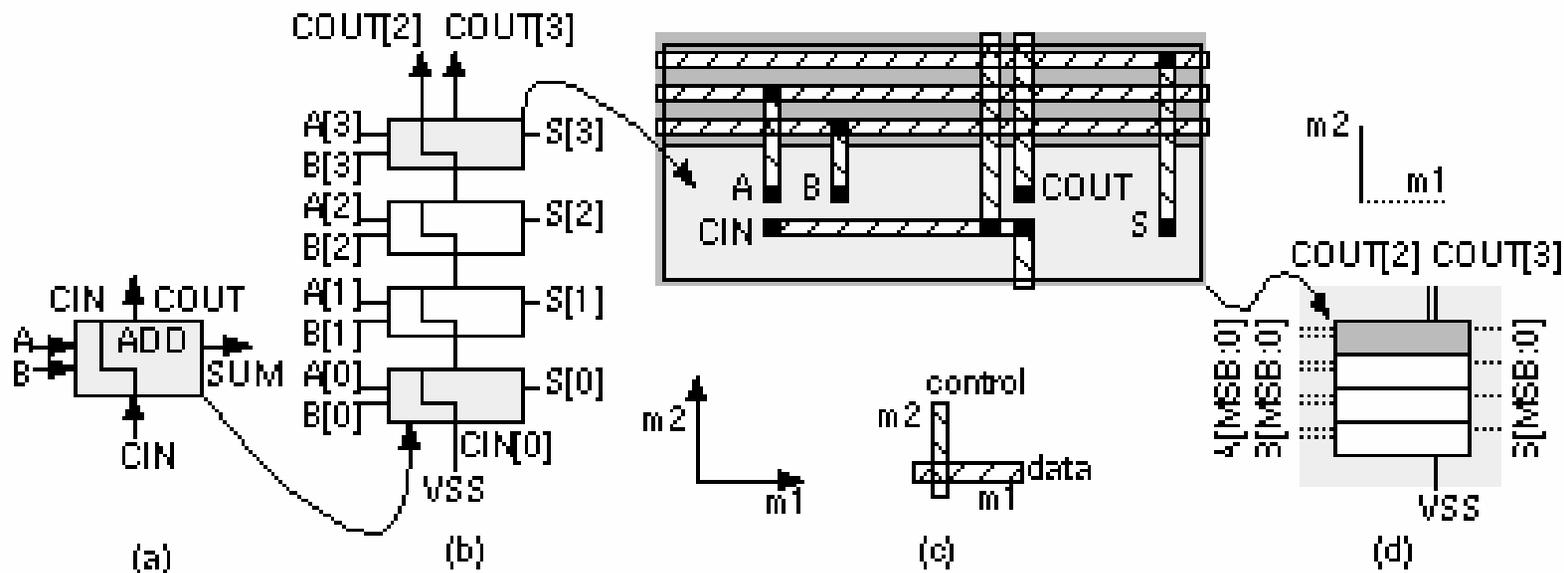
The layout of buswide logic that operates on data signals is called a Datapath.
