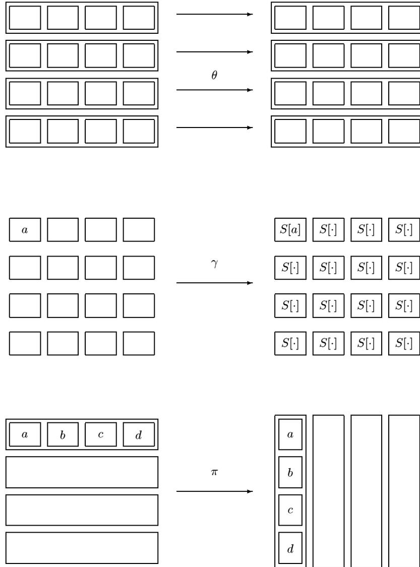
**Fig. 1.** Geometrical representation of the basic operations of SQUARE.  $\theta$  consists of 4 parallel linear diffusion mappings.  $\gamma$  consists of 16 separate substitutions.  $\pi$  is a transposition.
