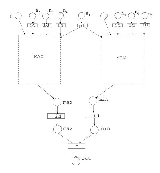
Figure 4.16: Schematic of PRES+ models for MINANDMAX-P source and transformed programs
