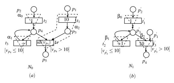
Figure 6.6: Illustrative example for the equivalence checking algorithm.
