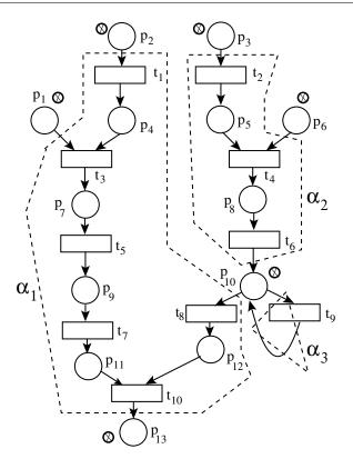
Figure 6.1: SCP Induced Paths of a PRES+ Model.
