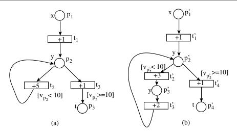
Figure 3.6: Computational equivalence of two PRES+ models.
