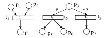
Figure 3.1: Places and transitions in a PRES+ model.
