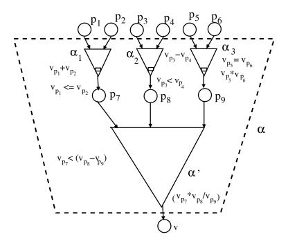
Figure 4.5: Concatenated Path of a PRES+ model.
