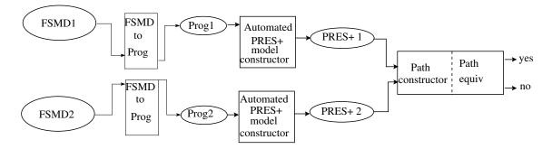
Figure 4.9: Experimentation using automated model constructor
