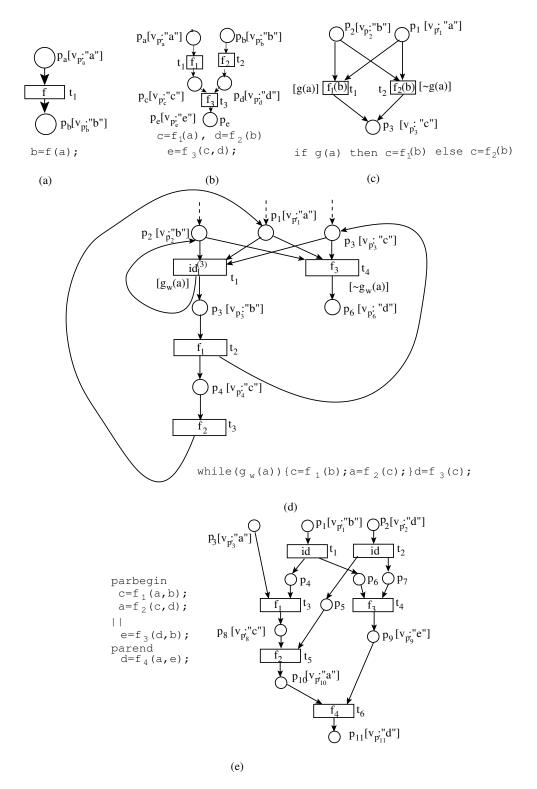
Figure 3.3: PRES+ model snapshots for various high level language constructs.
