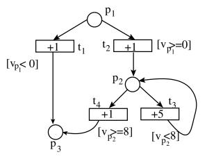
Figure 3.2: Computation in a PRES+ model.
