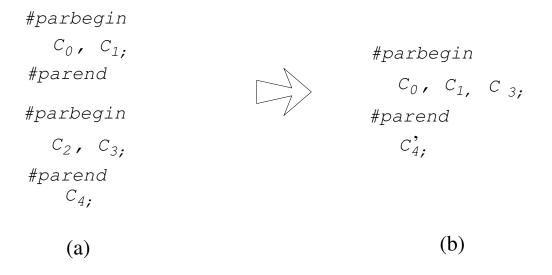
Figure 5.1: Code motion transformation for parallel programs
