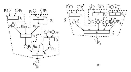
Figure 6.10: Initial and transformed behaviour of PRES+ models.
