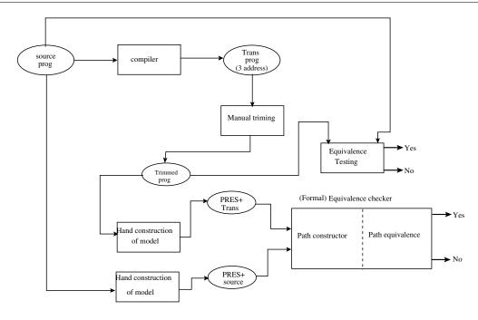
Figure 4.8: Experimentation using hand constructed models
