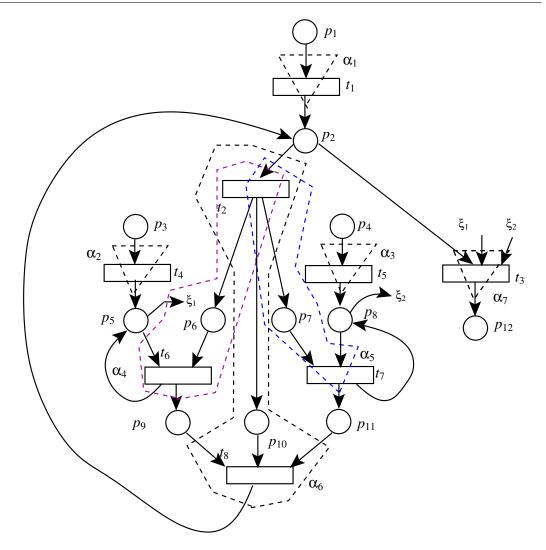
Figure 6.3: SCP Induced Paths of a PRES+ model.
