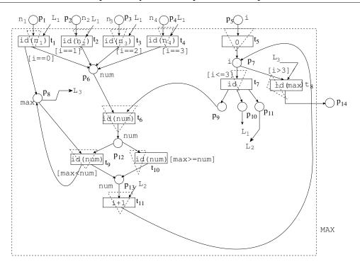
Figure 4.17: PRES+ subnet corresponding to MAX function
