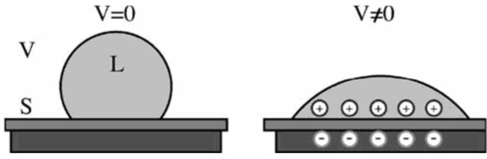
Figure – 4: Droplet changing its contact angle due to electrowetting.
