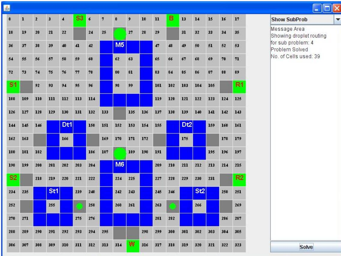
Figure – 18: The droplet routing simulation tool is showing the completion of subproblem 5 and number of cells used in routing.
