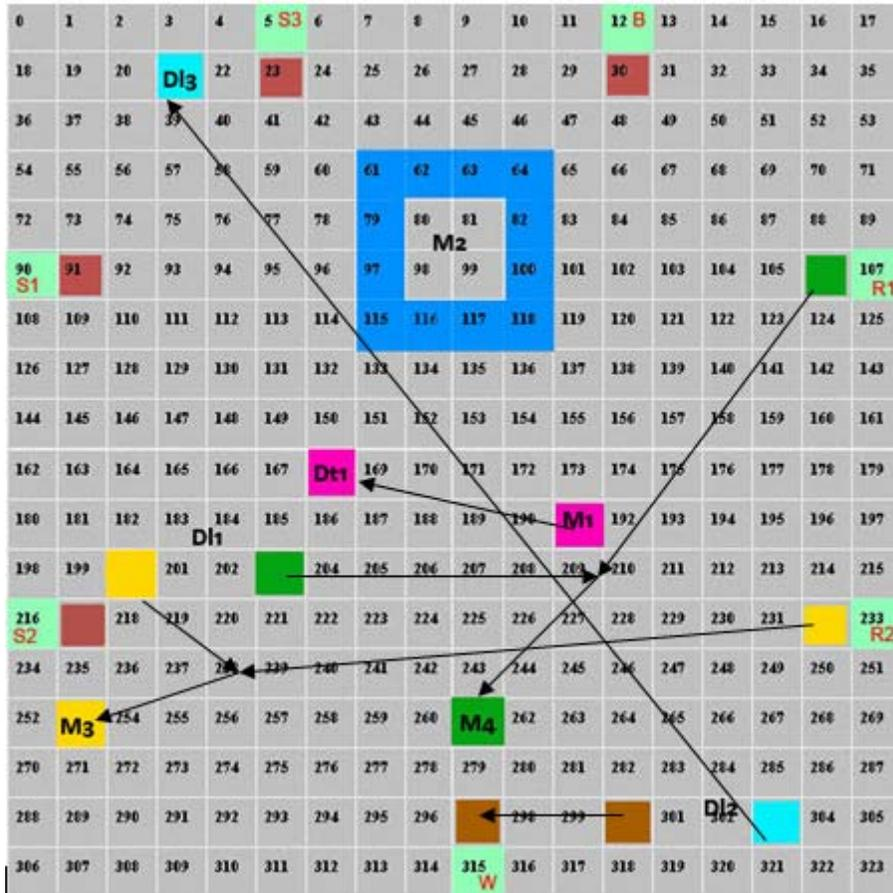
Figure – 15: Three 2-pin nets and two 3-pin nets to be routed in solving sub problem 3. Module M2 act as an obstacle while routing because it is active during that time interval.
