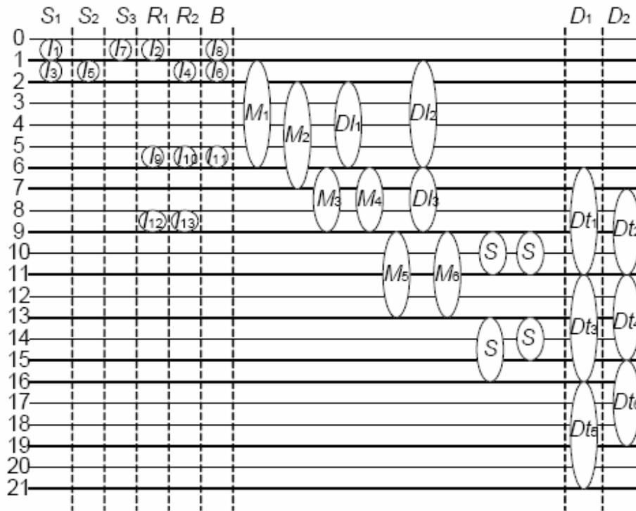
Figure – 10: Schedule obtained via architectural level synthesis
