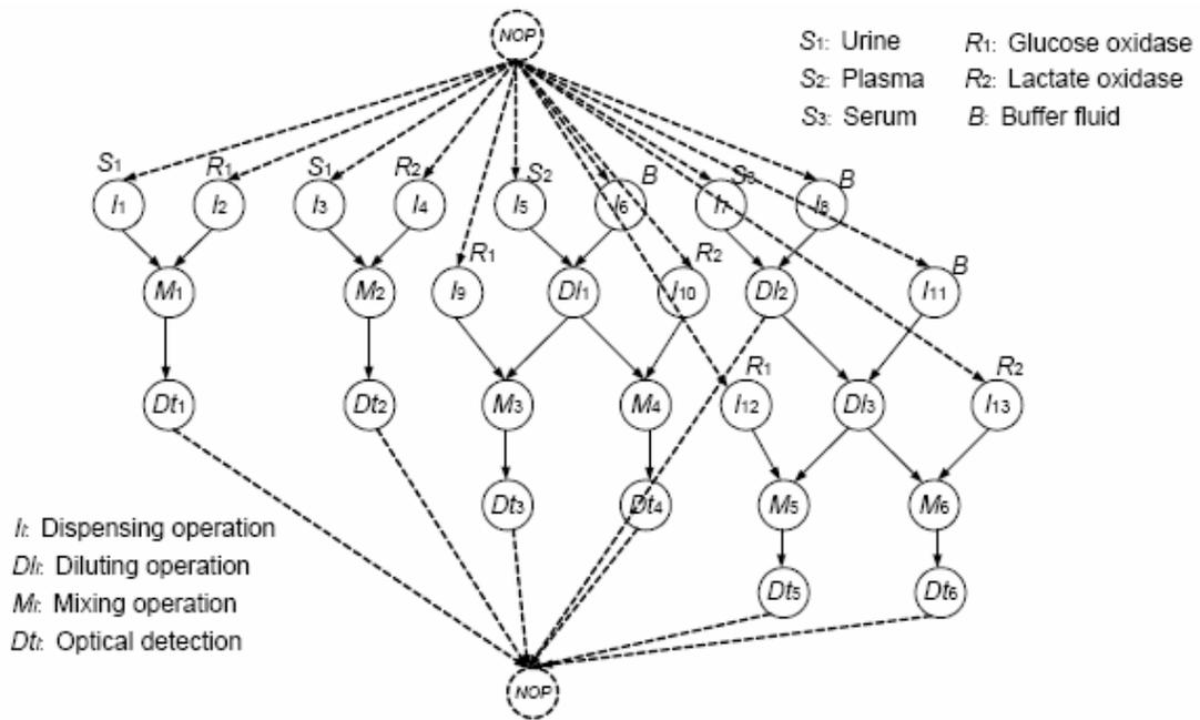
Figure – 8: Sequencing graph model of assay example
