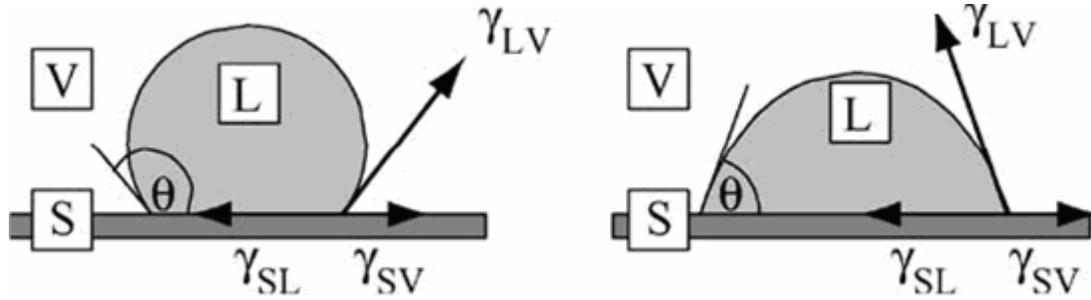
Figure – 2: Droplet on a substrate. Left: hydrophobic surface. Right: hydrophilic surface.
