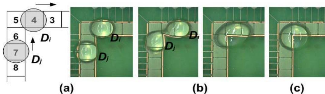
Figure - 13: (a) Experimental verification of Rule #3: droplets begin on electrodes 4 and 7; (b) Electrodes 3 and 6 are activated, and 4 and 7 deactivated; (c) Merged droplet.
