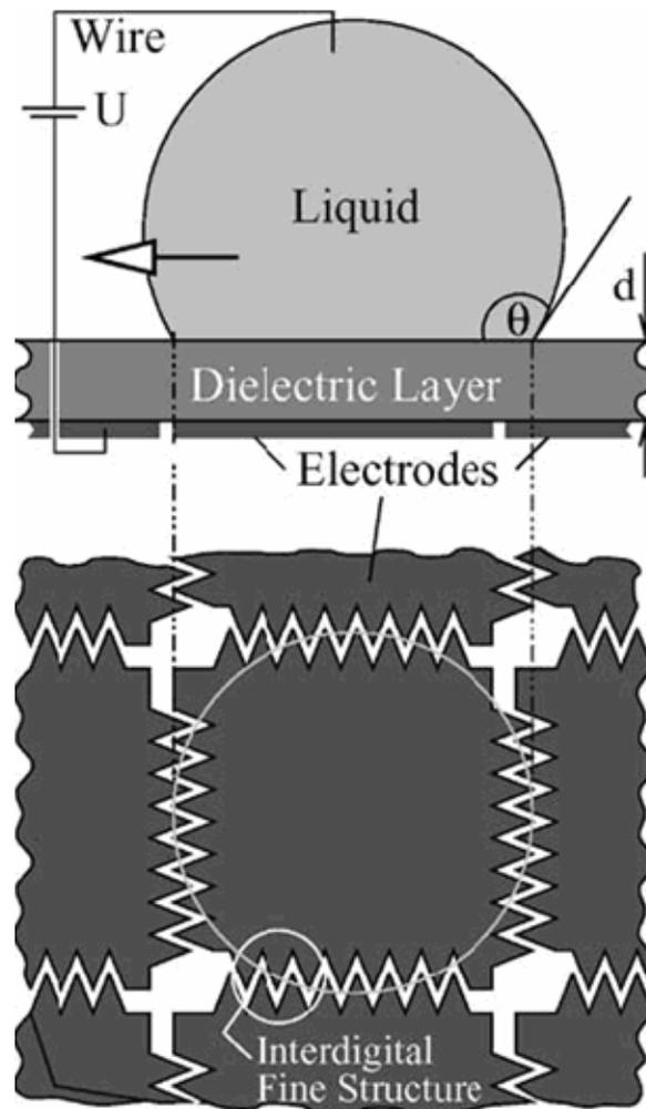
Figure – 3: Typical setup of an electrowetting device. The contact angle  $\theta$  is lowered if a voltage  $U$  is applied.
