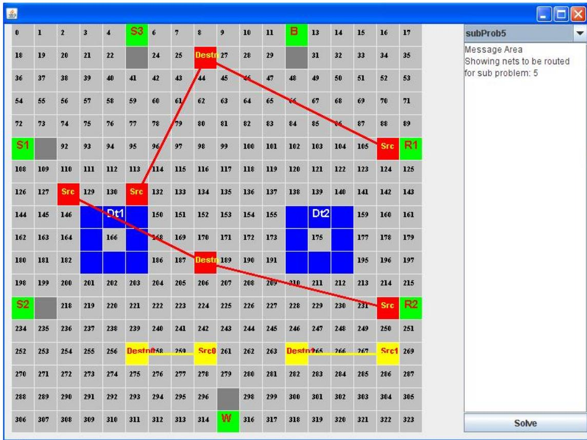
Figure – 16: The droplet routing simulation tool shows the nets to be routed for the subproblem 5.
