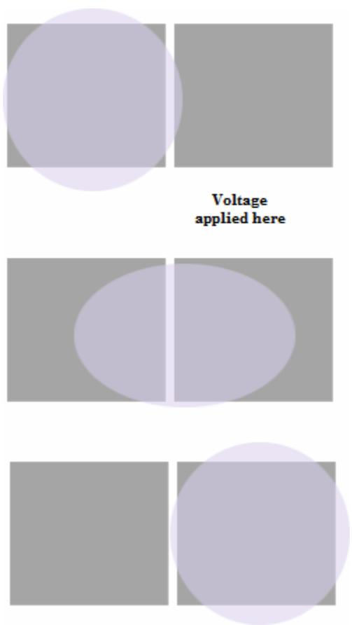
Figure – 5: Movement of Droplet to the next electrode
