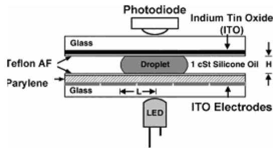
Figure – 7: An example of a basic unit cell used in colorimetric enzyme-kinetic assay
