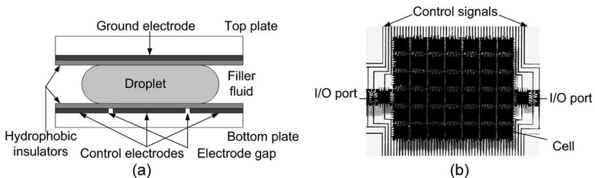
Figure – 6: Basic unit cell used in an EWOD-based digital microfluidic biochip; (b) a 2-D array for digital microfluidics. Control signals are used to control the electrodes.
