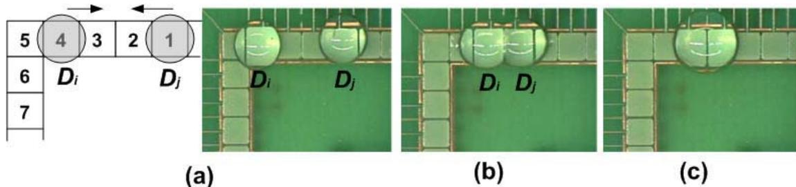
Figure 12: (a) Verification of Rule #1: droplets begin on electrodes 1 and 4; (b) Electrodes 2 and 3 are activated, and 1 and 4 deactivated; (c) Merged droplet.
