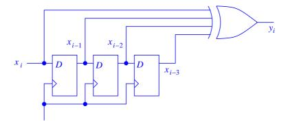
**Note:** The above circuit is a Mealy machine that assumes that the output is read immediately before the active edge of the clock pulse, that is, immediately before the state transition occurs. If you read the output *after* the state transition, a 4-bit shift register is necessary. Now, it is a Moore machine, so the output remains constant between two state transitions.
