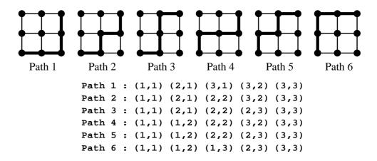
We print these paths using a stack. We initially push the point (1,1) to the top of the stack. Against every point in the stack, we maintain a direction indicator which implies the next direction to explore from this point: 0 means along x direction, 1 means along y direction and 2 means that both directions are explored from this point. Whenever we push a point, we set its direction indicator to 0. When the indicator becomes 2, we pop it from the stack.
